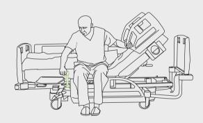
The patient can slide out the Mobi-Lift® handle using one hand.
