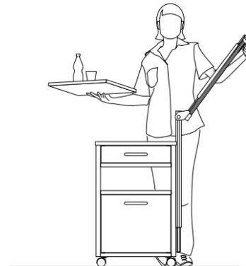
The overbed table is attached to the side and can be easily swung out with one hand, so that the nurse does not have to put the eating tray down.
